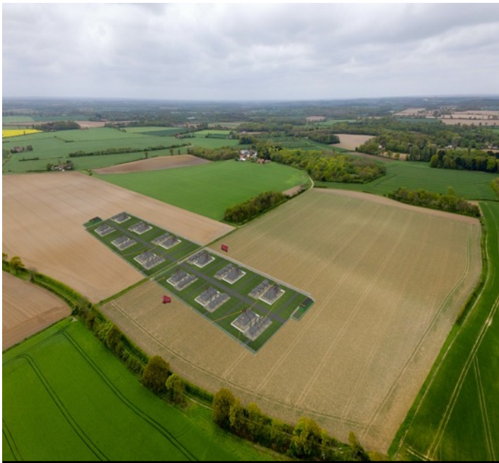
Visualisation of two cable relay stations (one north and one south of the loke) to scale, with approximate positioning on one of the proposed sites at Munn's Loke East Ruston. Note No decision as yet as to whether one or two stations would be built on the chosen site
